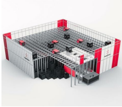
Fig. 1. Representative image of the AutoStore system
