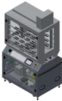
Fig. 5. Festo Didactic CP-F-ASRS32-P educational platform Source: Festo CP-F-ASRS32-P Manual [5]
