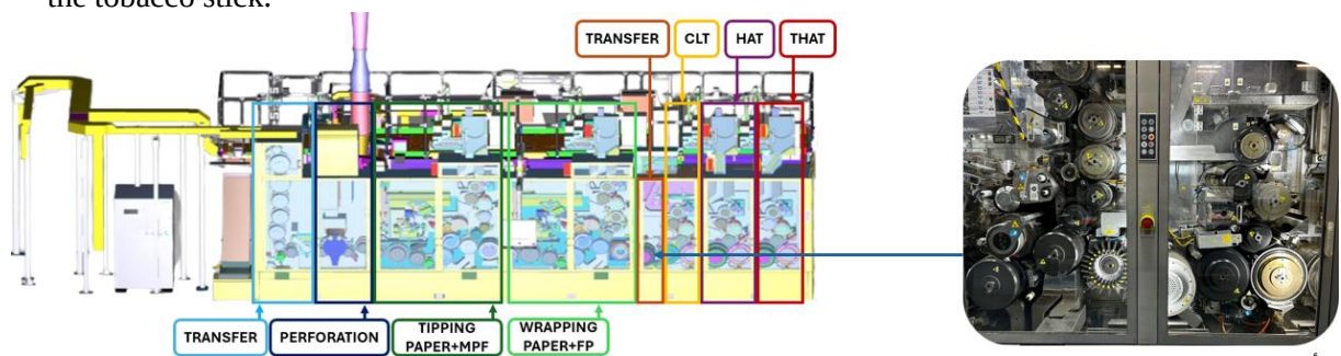
Fig. 3. Optical inspection area – location within the equipment
