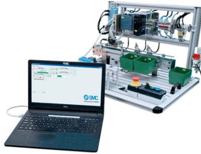
Fig. 6. SMC LOG-200 RFID Logistics Trainer platform Source: Website SMC International Training [6]
