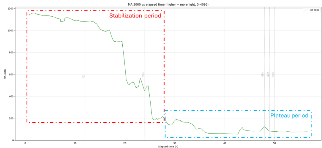
Fig. 4. ADC graph with 3000 moving average filter applied
