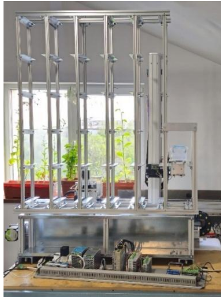
Fig. 8. Physically developed experimental AS/RS platform Source: own photography
