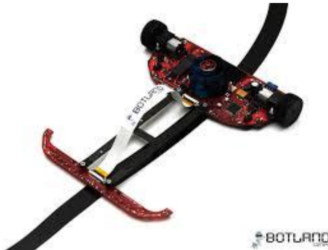
Fig 3. Example of a Line Follower robot equipped with a prebuilt EDF
