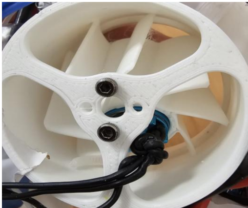
Fig. 10 heat based failure of the turbine
