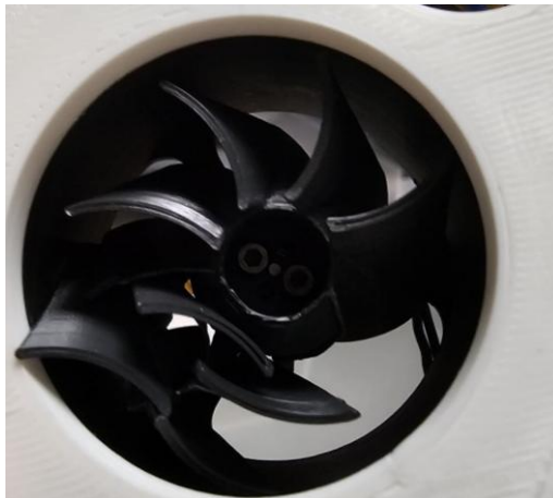
Fig.9 failure caused by exceeding centrifugal forces applied to ASA that split the turbine at layer lines
