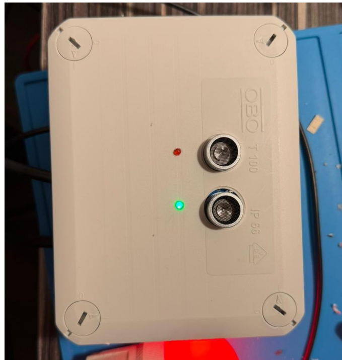
Fig. 4. View of the assembled functional prototype for water-level monitoring and smart irrigation
