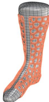
Fig. 5. Longitudinally sectioned Voronoi structure
