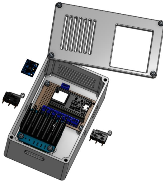
Fig. 6. Housing for the integration of the electrical components of the system
