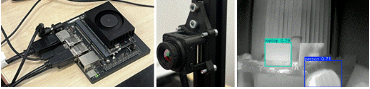
Fig. 3. Experimental setup: (left) NVIDIA Jetson Orin Nano edge node; (center) Thermal camera; (right) Real-time YOLO26n inference on the thermal stream.
