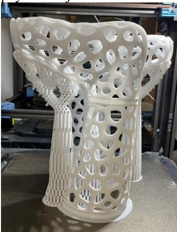
Fig. 7. 3D printed foot orthosis using the Sovol SV08 printer
