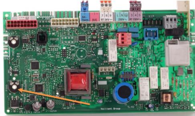
Fig.1. Boiler main board
