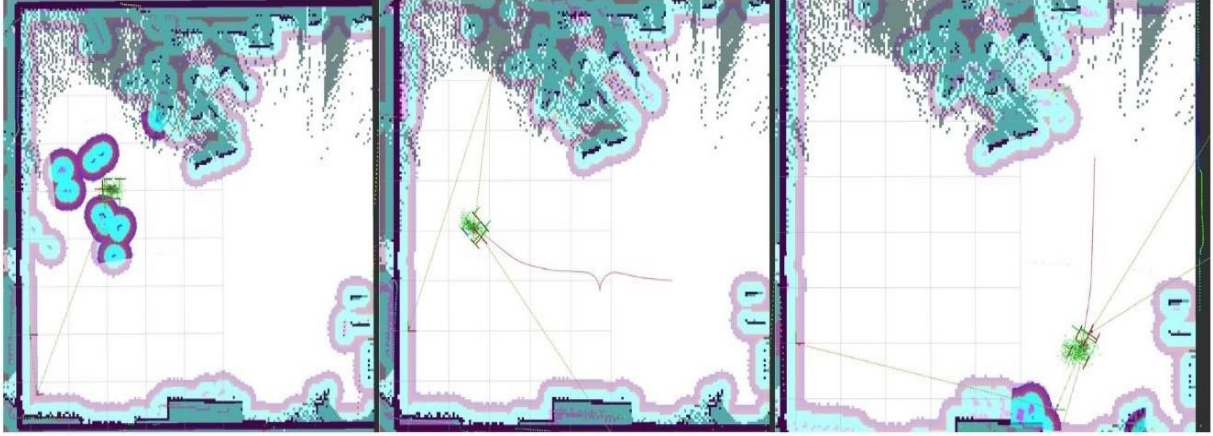
Fig. 2. SLAM-generated map of the test environment with a planned navigation path
