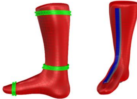
Fig. 9. Generation of the orthosis stability structure through a) rings and b) rails
