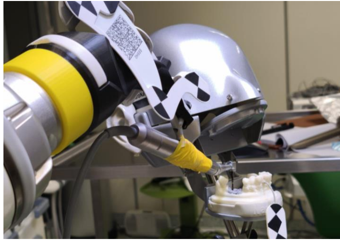
Fig. 2. Experimental setup for validating robotic instrument positioning
