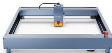
Fig. 2. xTool D1 Laser power: 5–10 W. Laser type: blue diode. Wavelength: ~450 nm. Spot size: ~0.08 mm. Materials: wood, plastic, leather, painted metal. Cutting area: ~300×300 mm. Cutting speed: high.
