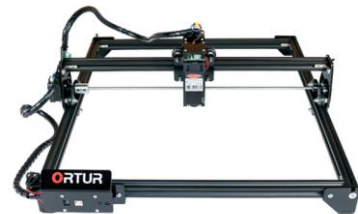
Fig. 3. Ortur Laser Master Laser power: 5–10W. Laser type: blue diode. Wavelength: ~450 nm. Spot size: ~0.06–0.1 mm. Materials: wood, leather, cardboard. Cutting area: ~400×400 mm. Cutting speed: high.
