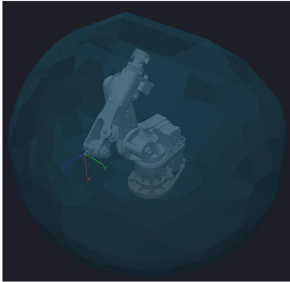
Fig. 13. Calculated effective workspace of the robot
