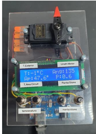
Fig. 4. The system built on the Arduino Uno platform, which provides automated climate control
