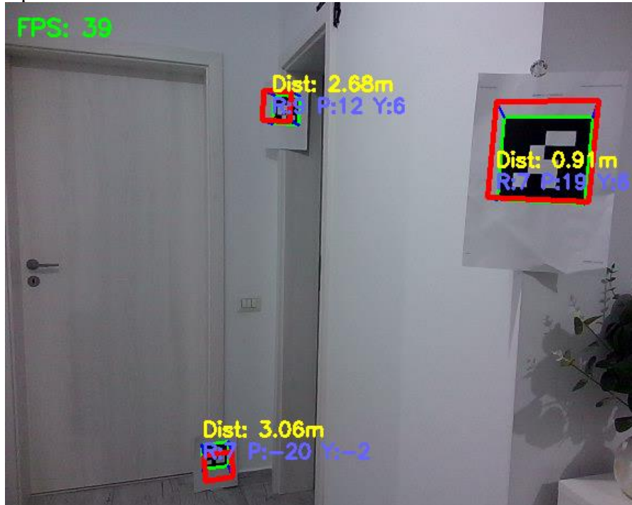
Fig. 4. AprilTag detection showing the 3D wireframe and the "FPS: 39" indicator.
