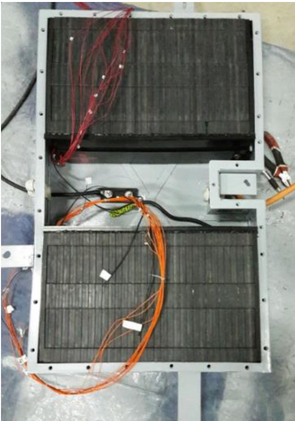
Fig. 7 Module asamblate, fixate in incinta si cablate
