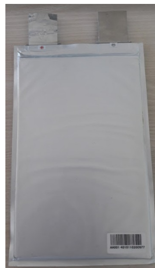
Figura 2.4.1 Celula Lithium-Ion 3,65V 40Ah
