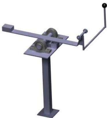
Fig. 9 Model opritor manual
