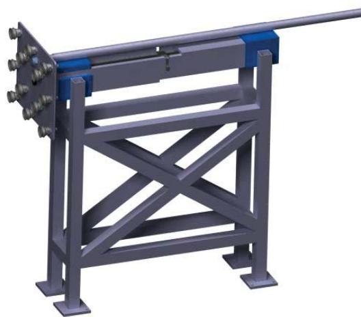
Fig. 12 Sistem vacuumatic de incarcare/descarcare
