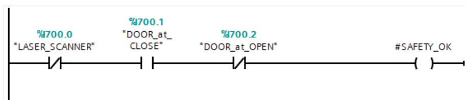
Fig. 10. Bloc de program SAFETY
