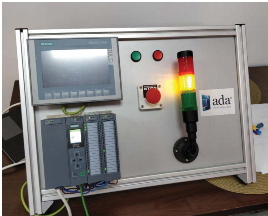
Fig. 9 Stand ce contine PLC Simatic S7 1500, Interfata HMI, semafor indicator si butoane de actionare.
