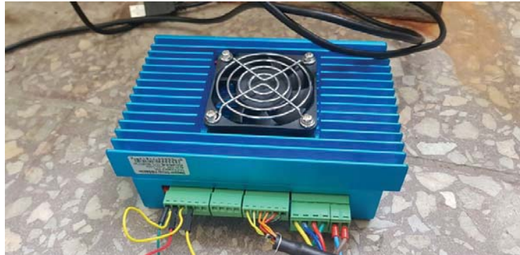
Fig 13 – Placa de control HBS860H
