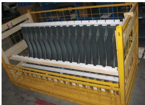
Fig.12 Piese conditionate in ambalaje metalice
