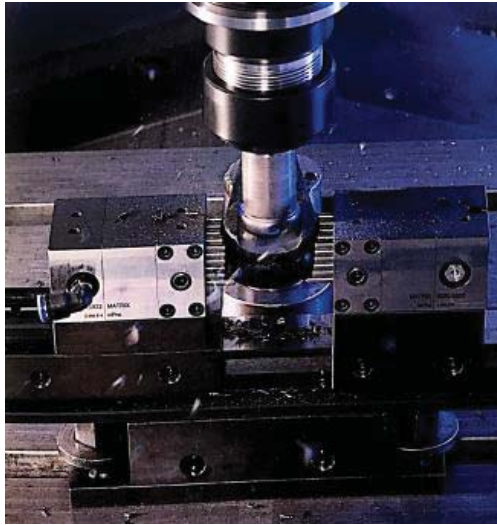
Fig 17 Frezare piesa prinsa in sistemul SILVER CLAMP
