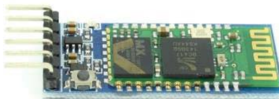
Fig.3. Modul Bluetooth HC-05
