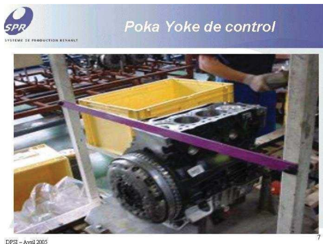
Fig. 5 Poka Yoke de control
