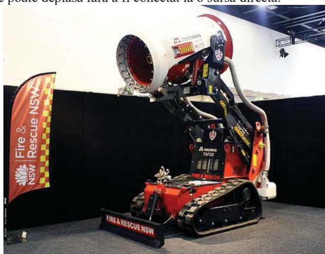
Fig. 3. Turbine Aided Firefighting Machine
