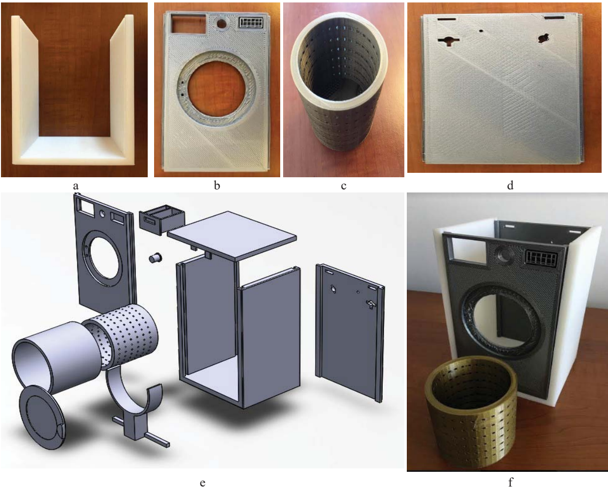
Figure 2. The 3D printed components of the washing machine
