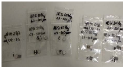
Fig. 12. Halved AlSi10Mg samples (20-63 μm and 63-105 μm)
