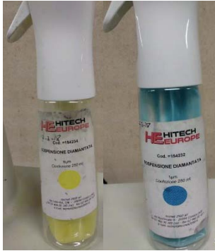
Fig. 19. Diamond suspension (particle size of 6µm and 1µm)
