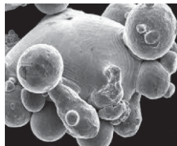
Fig. 8. Satellites attached to metal grains [3]
