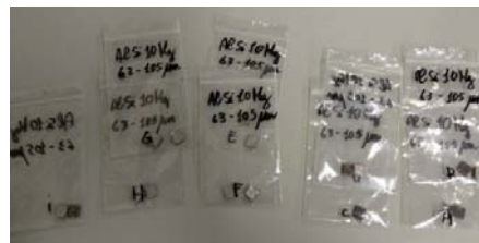
Fig. 12. Halved AlSi10Mg samples (20-63 μm and 63-105 μm)
