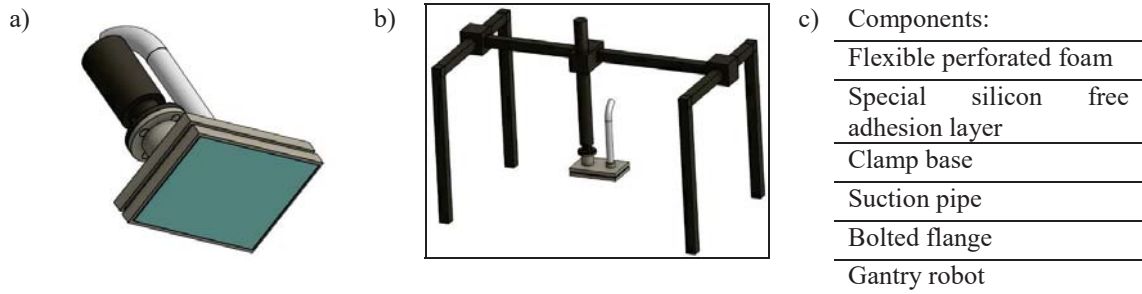
Figure 5: (a) 3D model of concept 2 (b) positioning of the product on the Gantry robot (c) List of main components
