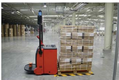
Fig.3. Stivuiitor Smart Laser forklift AGV transfer robot X14-L01 Series
