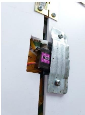
Fig. 15 Detaliu prindere servomotor
