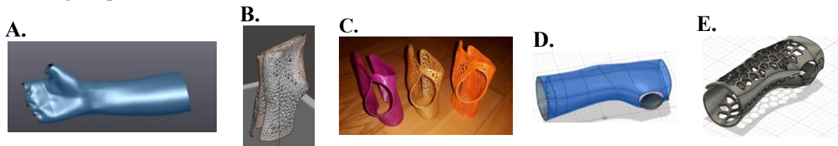
Fig. 1 Transformation stages of the orthosis
