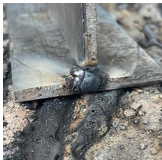
FIG. 2.3.3. REMOVING SLAG WITH A HAMMER
