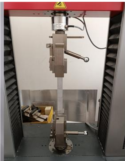
Fig. 8. Zwick Roell universal testing machine with aluminum-aluminum test specimen fitted for tensile testing.
