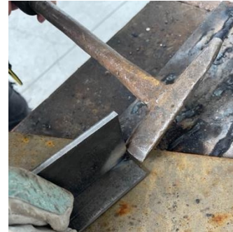
FIG. 2.3.2. FIXING PARTS BY SPOT WELDING
