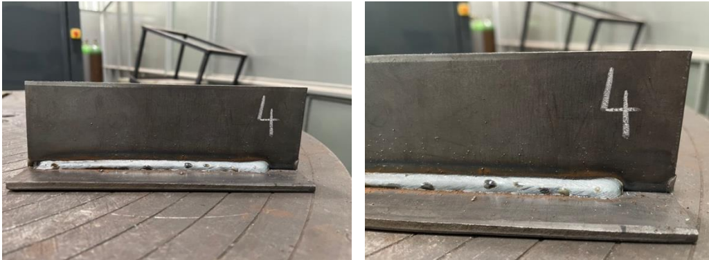
FIG. 2.4.4. WELDED JOINT SAMPLE 4
