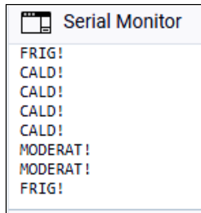
Fig. 14. Messages sent to the Serial Monitor by the temperature sensor
