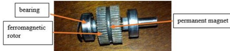
Fig. 2. Rotor of a hybrid stepper motor (laboratory motor).
