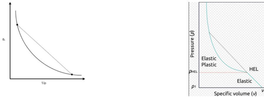
a. Hugoniot and Rayleigh shock line in p-v plane for weak shock b. Hugoniot elastic limit in the p-v plane for shock in the elasto-plastic field
