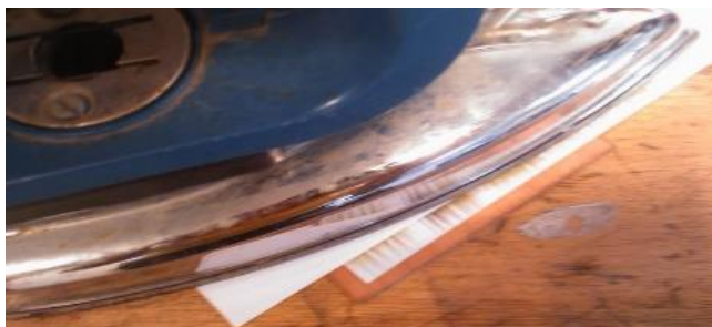
Fig. 10. "Ironing" the PCB
