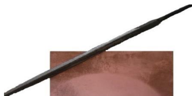
Fig. 8. Filing PCB edges
