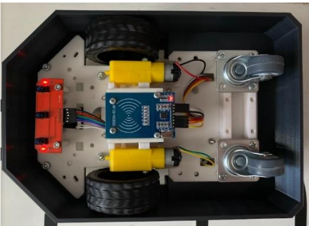
Fig. 8. Lower part of the physical model highlighting the sensors used
