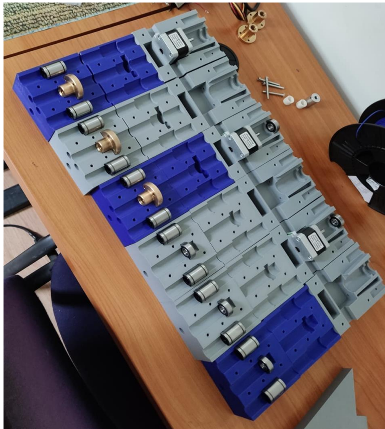
Fig.5. Resulted 3D printed parts with components slotted in
