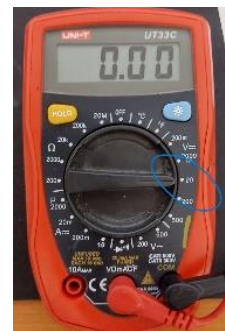
Fig.27 DC voltage measurement
