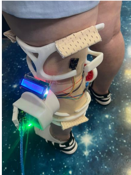
Fig. 9. Wearing orthosis functional prototype
