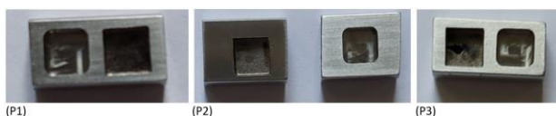
Fig. 9 Parts of CoCr alloys processed by EDM and milling
