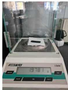
Fig.3. Weighing samples at precision analytical balance 10-4 g
