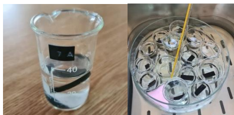
Fig. 4. Place samples in distilled water according to the established procedure and keep at a temperature of 23 ° C in a thermostated water bath
