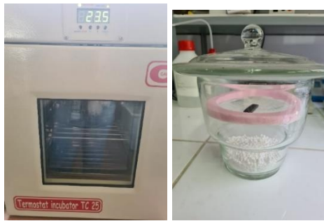
Fig. 2 Conditioning samples at 50 °and drying in a desiccator, with CaCl 2 as the moisture removal agent in the enclosure
