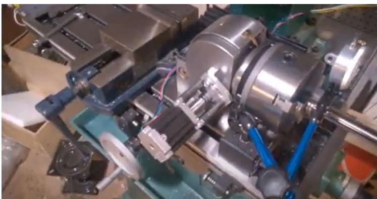
Fig. 5. CNC indexing head [9]
