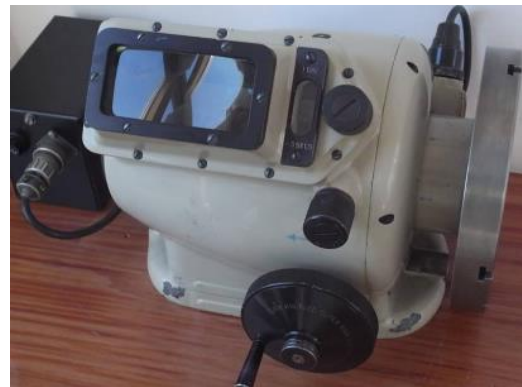
Fig. 4. Optical divider head [5]
