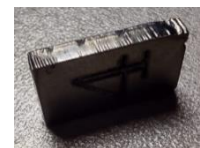
Low speed v=70 mm/s P=1000 W
