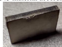
Increased speed v=80 mm/s P=1000 W
