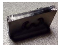
Increased speed v=90 mm/s P=1000 W
