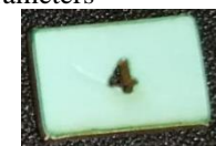
Increased speed v=17 mm/s P=78 W
