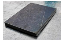
C45 2mm v = 4350 \text{ mm/min} p = 5 \text{ bar} I=35A (P = 13.3 \text{ kW})
