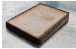
Inox 4mm v = 3500 \text{ mm/min} p = 5.6 \text{ bar} I=45A (P = 17.1 \text{ kW})
