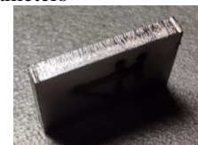
Low speed v=60 mm/s P=1000 W
