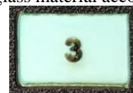
Low speed v=10 mm/s P=78 W
