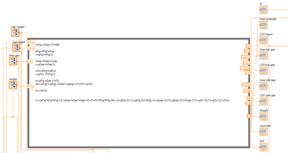
Fig. 5. Formulas implementation using Formula Node
