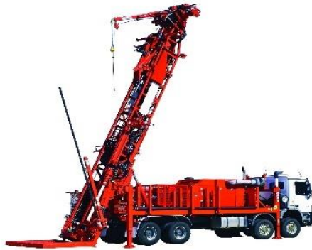
Fig.2. The loading equipment for drill rods.
