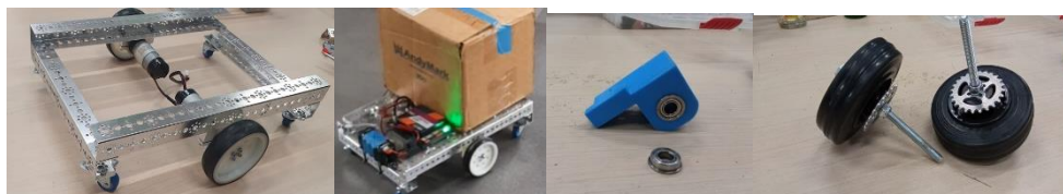
Fig. 7 Switching from wheel locations directly on the drive shaft to the use of a gear and chain gear
