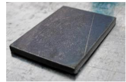
C45 2mm v = 4350 \text{ mm/min} p = 5 \text{ bar} I=35A (P = 13.3 \text{ kW})
