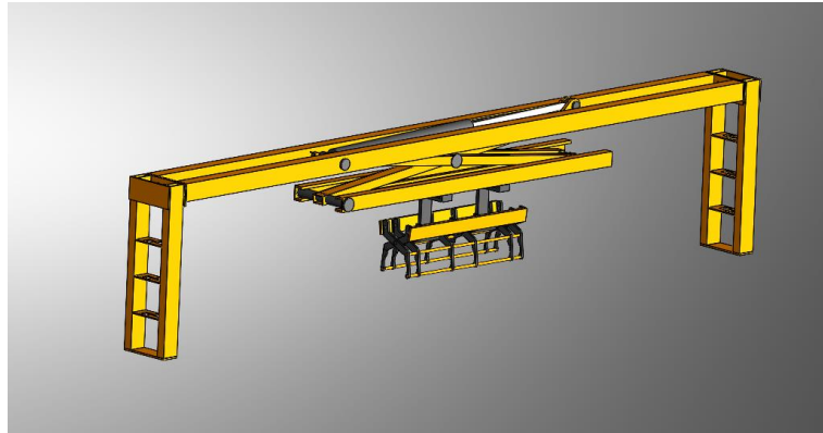
Fig. 7. The 3D model of the bridge crane
