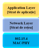
Figure 4 – ZigBee Protocol Stack
