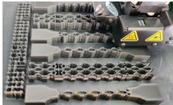
Fig. 10. Test pieces on the table of MARKFORCED machine
