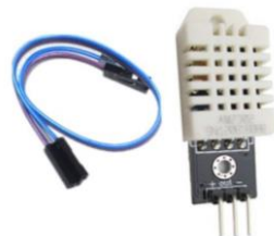
Fig. 6. DHT22 temperature and humidity sensor
