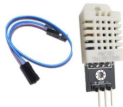
Fig. 6. DHT22 temperature and humidity sensor
