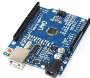
Fig. 5. Arduino compatible UNO R3 development board
