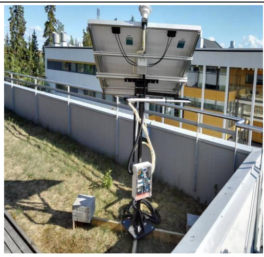
Fig.4. Solar tracker with two axes and online energy monitor[5]
