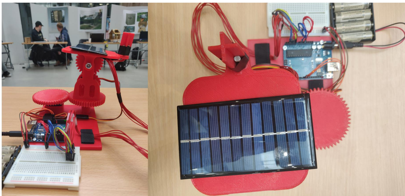
Fig.2. 3D printed dual axis solar tracker
