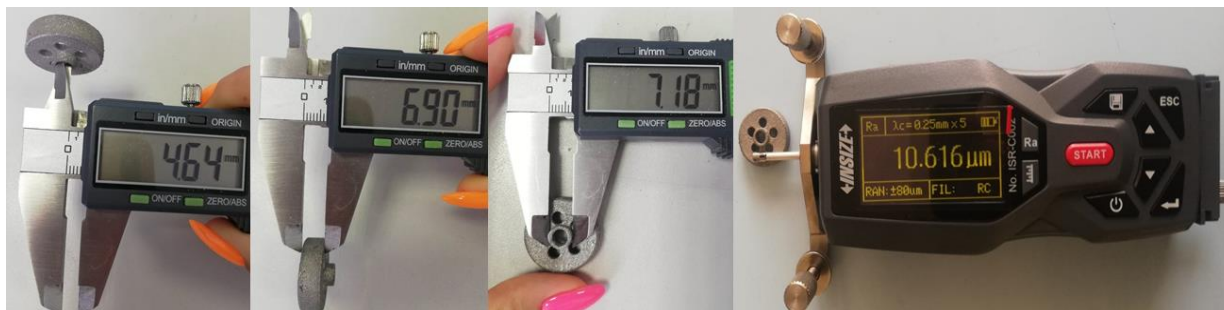
Fig. 7 Dimensional verification of the part
