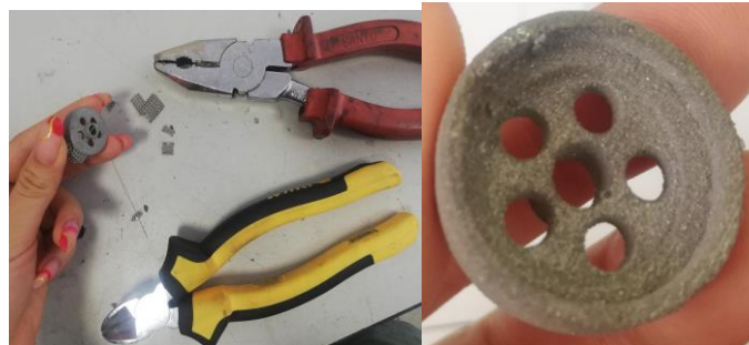
Fig. 6 Removing supports and final part
