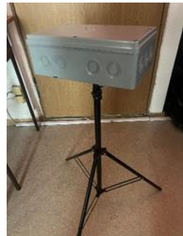
Fig. 3 - Temperature and humidity measuring stand
