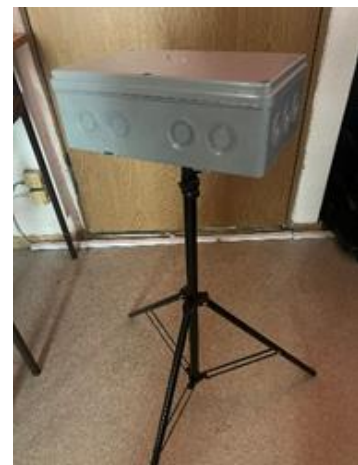
Fig. 3 - Temperature and humidity measuring stand
