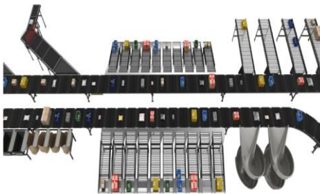
Fig. 1. Interroll MX_H horizontal sorter [1]
