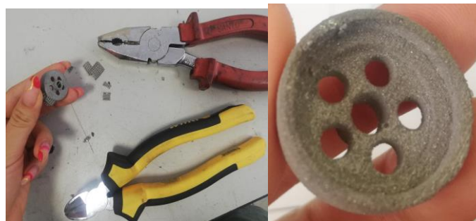
Fig. 6 Removing supports and final part
