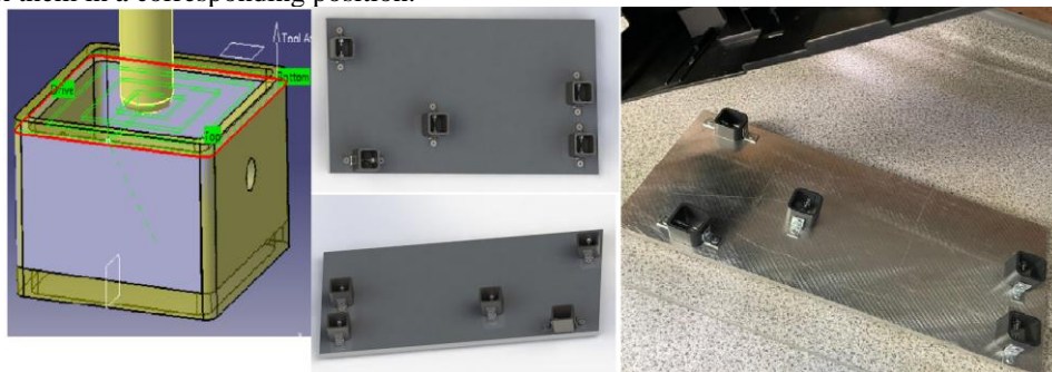
Fig 2.3.1- Device for fixing the part, CAM, rendered, real life
