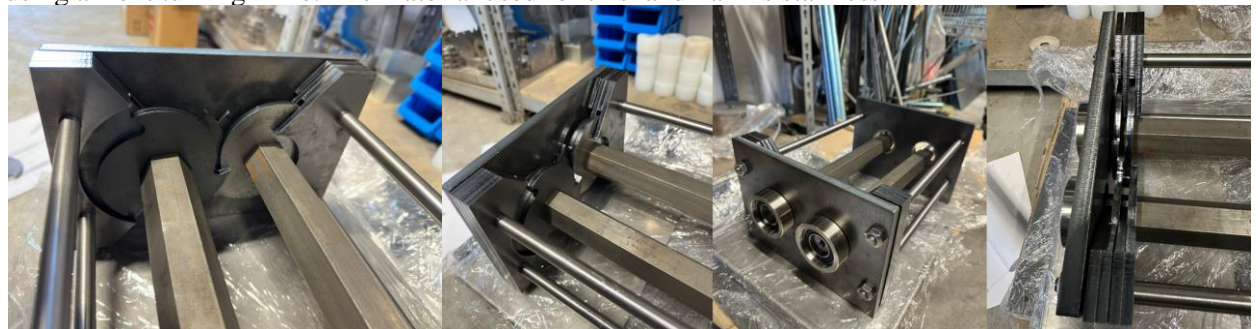
Fig. 1.13. Trial assembly of the chopping mechanism subassembly
