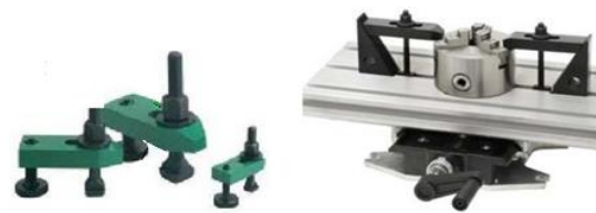
(b) Clamping with force elements type of nut - washer – screw - clamp at various devices
