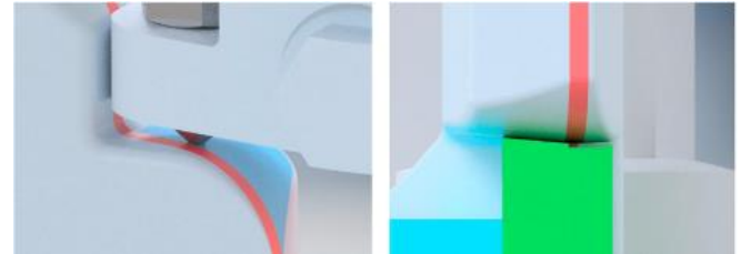
Fig. 13. Fixing the part with dog point screws for reducing the contact area and the appearance of deformations [10]
