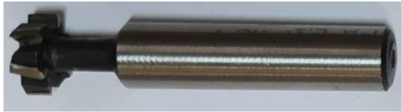
Fig. 5. Side mill used for machining eccentric channels [4]
