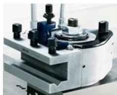
(a) Clamping with force elements type of screw - threaded hole within lathe tool holder
