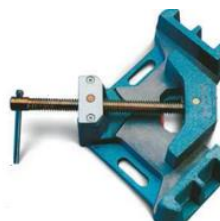
(c) Clamping with force elements type of screw - fixed nut -jaws, at vises and other devices
