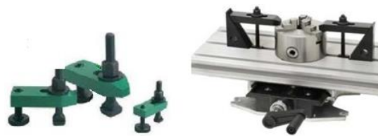
(b) Clamping with force elements type of nut - washer – screw - clamp at various devices
