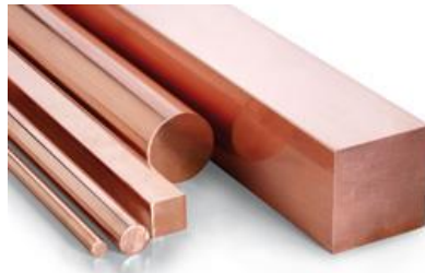
Fig. 4 Shapes of tool-electrode
