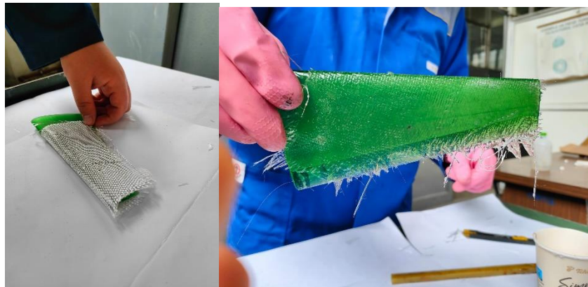
Fig. 5 – the physical figure before and after glueing the fiberglass
