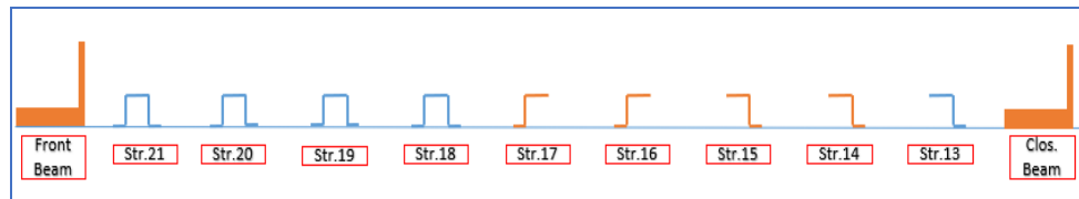
Fig. 5 Sequence of stiffeners along HS skin panel.
