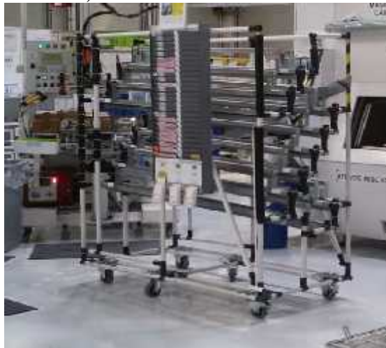
Fig.7 Intermediate subassembly storage space
